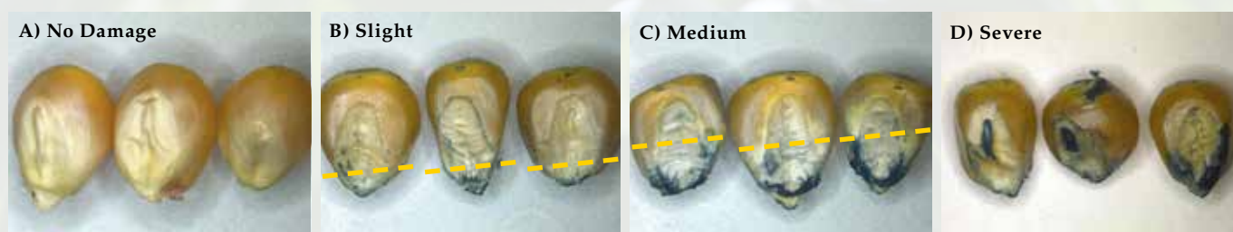
FIGURE 2. Pericarp Damage Test: A) None: no visible damage to pericarp covering, B) Slight: tearing of pericarp area extending up less than 25% length of embryo pericarp margin/edge, C) Medium: tearing of pericarp extending up to 50% of length of embryo pericarp margin/edge and D) Severe: cracks over the embryonic axis and major breaks in seed or missing parts of the seed.
