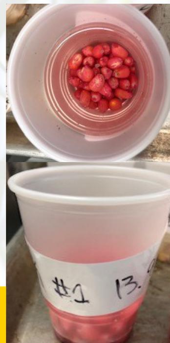
**FIGURE 2.** 50 corn seeds soaking in 75 ml of deionized water.
