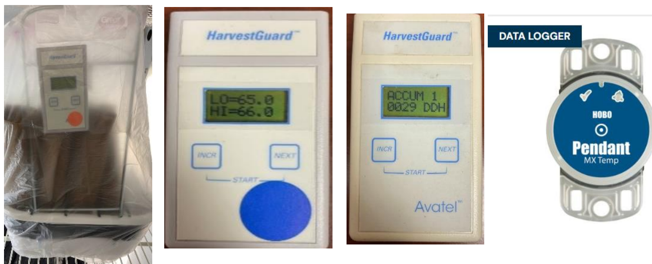
Figure 1. From left to right: Inner chamber prototype with HarvestGuard™, close-up of HarvestGuard™ showing Low/High temperatures, GDDs and an Onset® Pendant®. (The abbreviation DDH use by Avatel™ means Degree Day Hours. Avatel™ uses the standard methods for calculating degree-days required by most current phenology models.)
