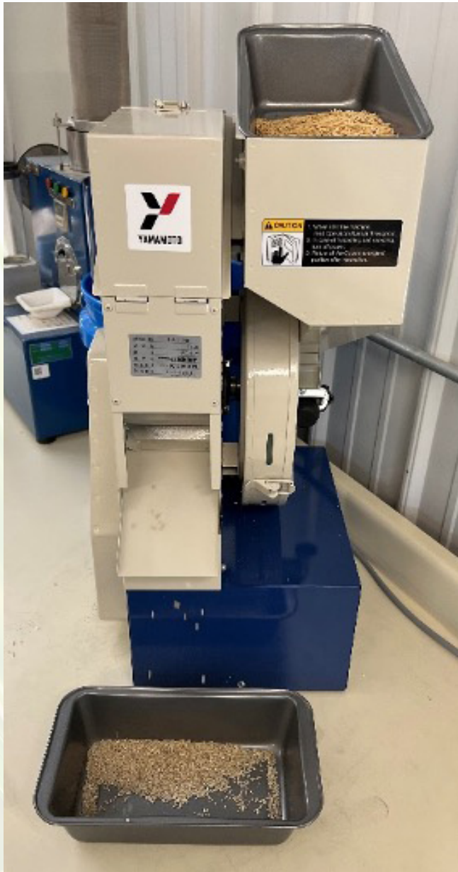
FIG. 6. A rice dehuller mill is used to remove hulls prior to a red rice exam.
